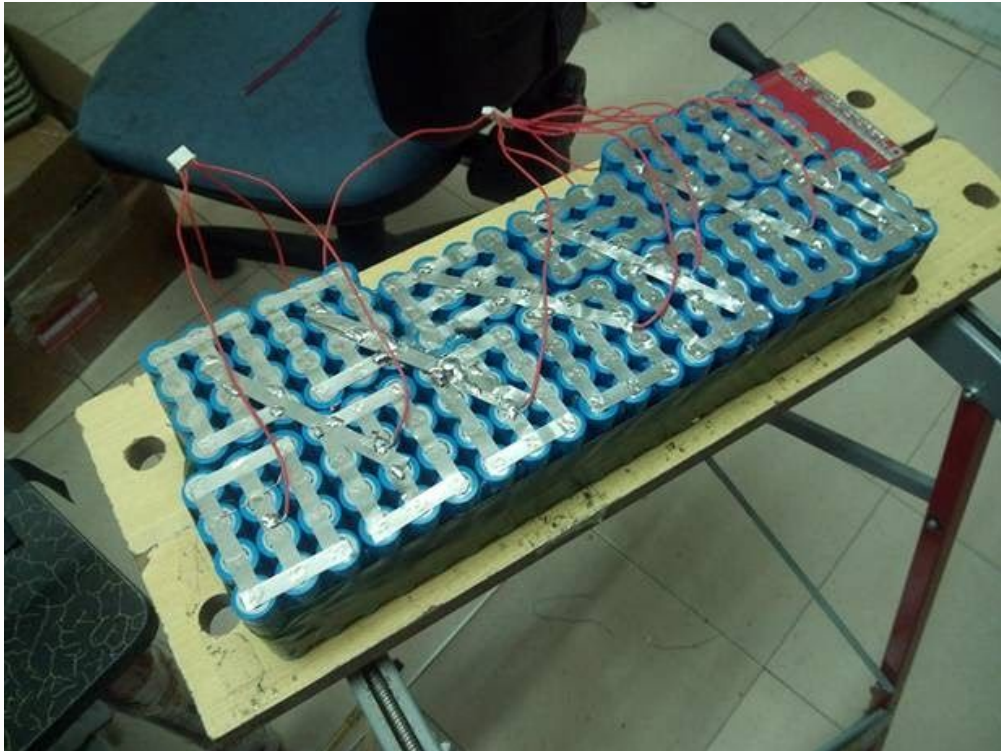
EV Battery pack use the DC spot welding machine from customers
