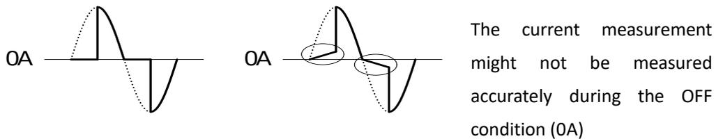
The actual current waveform      The abnormal current waveform
