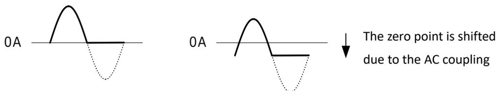
The actual current waveform      The AC coupled current waveform
