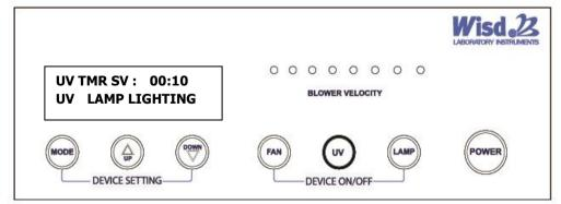
The timer setting time range of UV Lamp is 00:00 thru 99:99 (99hr and 99min), and 00:00 means the continuous operation.
