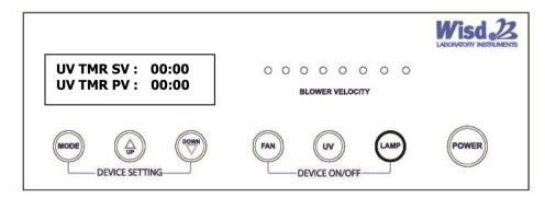
The Lamp is operated to ON/OFF by touching "LAMP" button.
