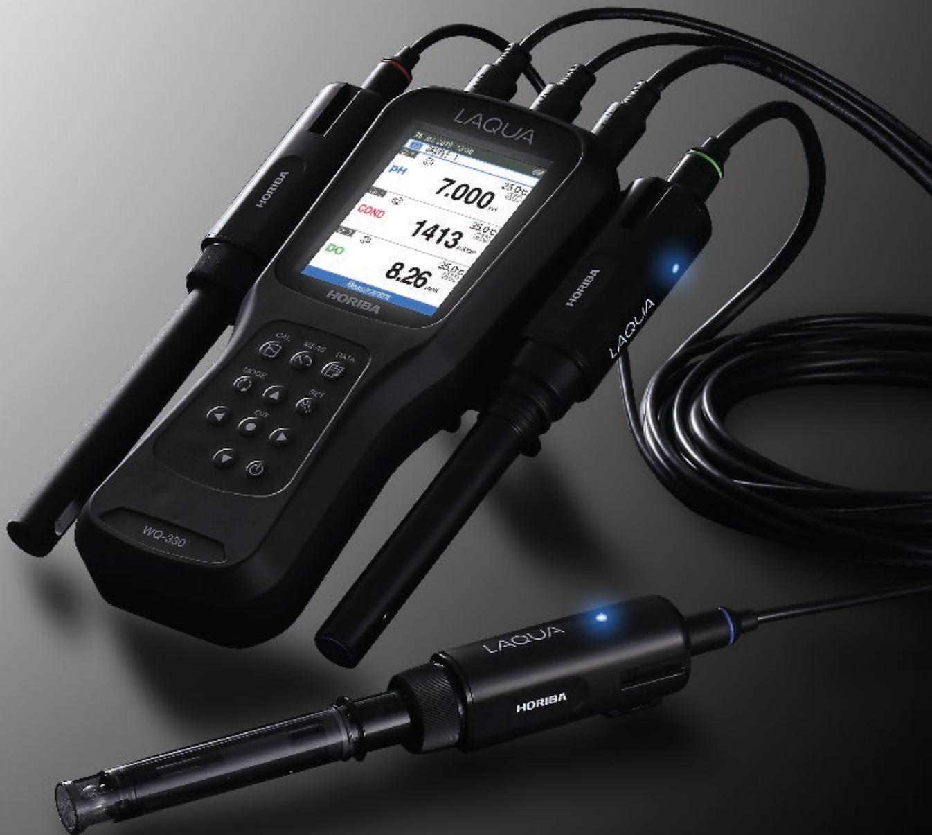
pH | ORP | Dissolved Oxygen | Conductivity | Resistivity | Total Dissolved Solids | Salinity | Ion
