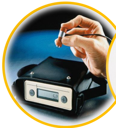
First Generation PosiTector 100 (1993) Primarily Intended for thicker coatings on concrete and wood
