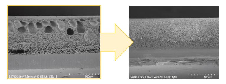
Existing (left) and new optical grade replica tape for improved resolution (right)
