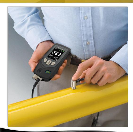
It is often critical to measure the effects of corrosion or erosion on tanks, pipes or any structure where access is limited
