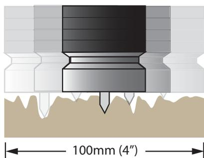
1. Ensure probe is 90° to substrate to ensure accurate readings and calibrate the gauge on a glass zero tile.
