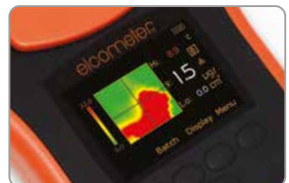
2D Salt Density Map with High/Low Readings
