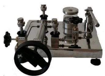
it calibrated 2pcs pressure instruments once. It is used widely to calibrate pressure transmitter,
