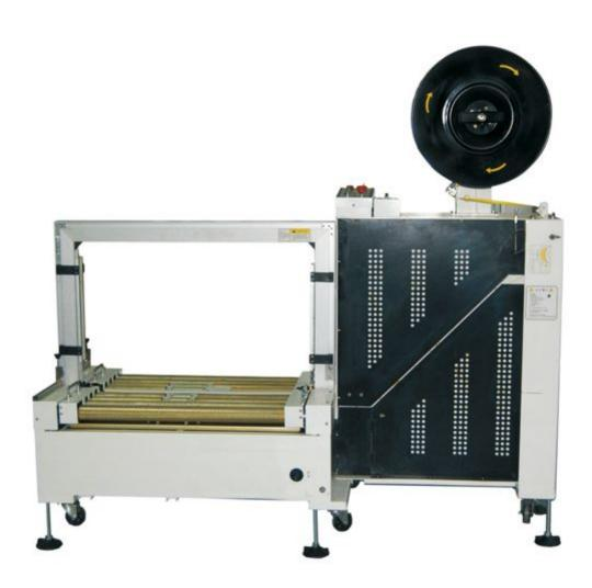
MH-102B low platform unmanned packing machine is suitable for the use of low surface assembly line. The platform is equipped with 8 dynamic galvanized embossing rollers, which can automatically detect, automatically pack and automatically transport, and the roller's embossing treatment increases the friction force at the time of residence, and makes the packing position more accurate. Widely used in food, chemical, clothing, post, logistics and other industries.
