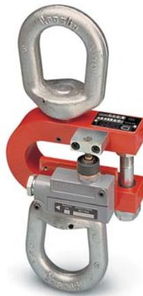
The heart of the system is a force beam which operates in tension or compression. Seven different load capacities are available. Switch and physical connection options are listed. Each beam can accommodate from one to four switches which can be set to operate as many as four different switching functions or combinations including slackline detection.
