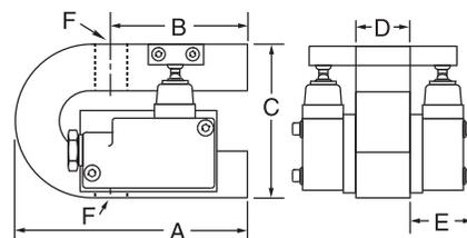
2,000 lb and 10,000 lb capacity force beam. Illustrated with two weatherproof switches (option 2).
