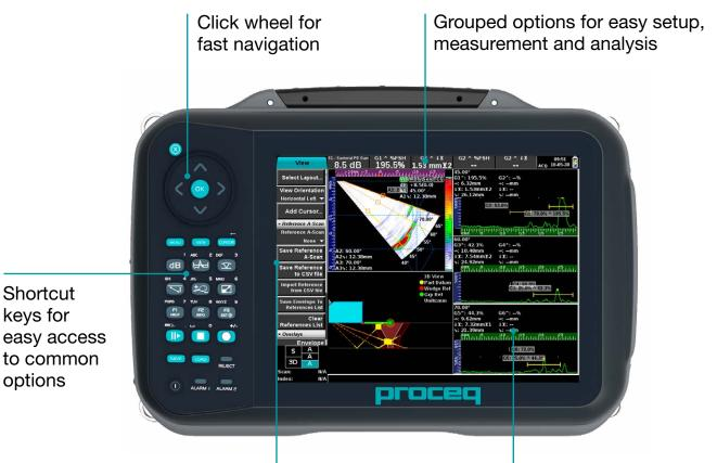
Context sensitive help and workflow based tabs provide an intuitive user interface Customizable screen with selectable layouts
