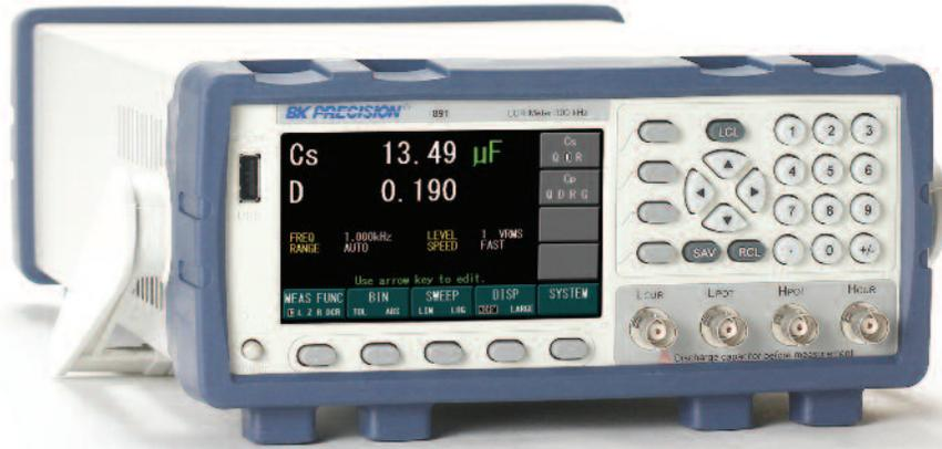
The 891 is a compact, precise, and versatile LCR meter capable of measuring inductors, capacitors, and resistors at DC or from 20 Hz to 300 kHz. The instrument's 2U half-rack form factor is suitable for the bench or rack mount installation. A large color display with all important parameters and measurements visible on one screen makes this meter easy to operate.
