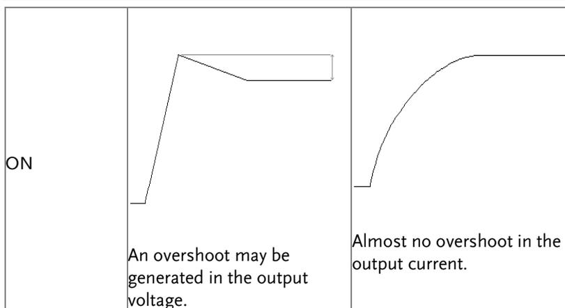
The above voltage and current waveforms assume that the resistance is the load of this unit.
