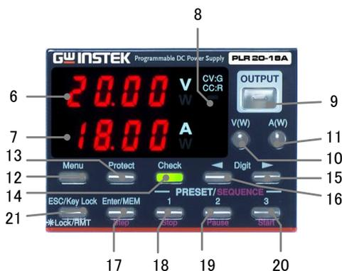
Operation Panel (The above figure shows the operation panel of the PLR 20-18)
