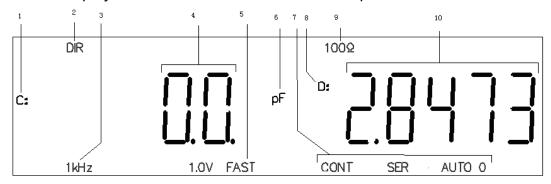
Figure 3.1 LCD Display in Measurement Status
