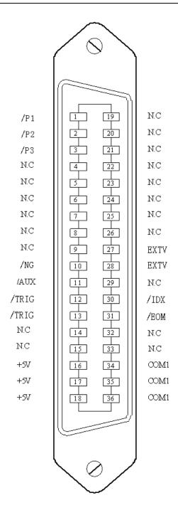
Figure 4-2 Pin Assignment for Handler Interface Connector
