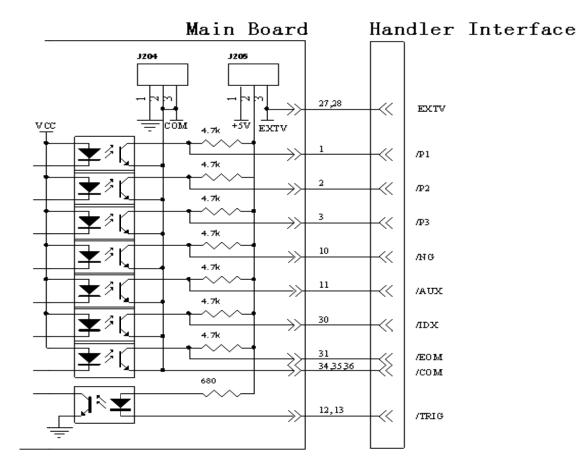
Figure 4-4 Simplified Diagram of output and control signals
