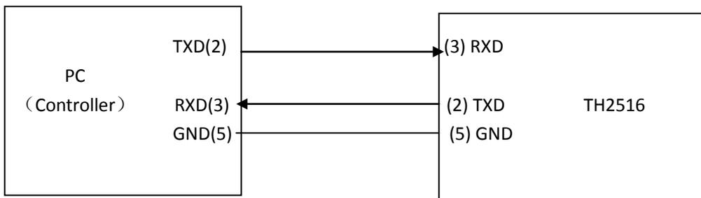
Figure 6-1 Connection of the instrument with PC
