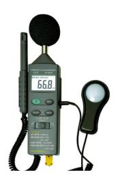
schools, offices, home, etc, checking acoustics of studios, auditoriums and hi-fi installations. The Light function is used to measure illuminance in the field. It is fully cosine corrected for the angular incidence of light. The light sensitive component used in the meter is a very stable, long life silicon ciode. The Humidity/Temperature uses a humidity/semiconductor sensor and K type thermocouple.
