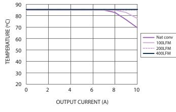
Figure 1 - Safe Operating Area Vin = 5 V, Output Voltage = 3.3 V (See Note A)
