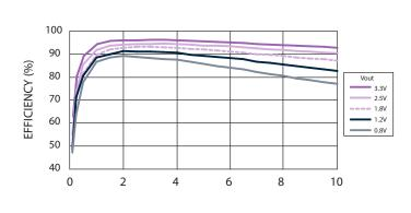
Figure 3 - Efficiency vs Load Current Vin = 5 V (See Note B)
