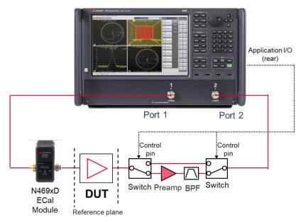
For calibration, a standard mechanical cal kit or ECal module is required for the S-parameter portion of the cal (an ECal used as a tuner cannot be shared for calibration). To calibrate a standard receiver for noise figure measurements, a power meter is required. All calibration accessories and external hardware must be ordered separately.
