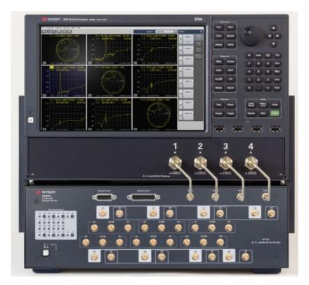
Figure 1. Multiport setup using the E5092A
