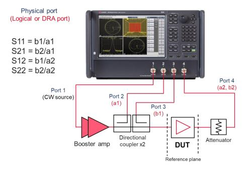
External components should be selected based on their high-power limits or frequency range specifications. Be sure that these components can handle the output power level of the booster amplifier.
