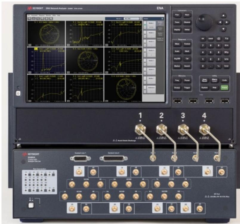
Figure 1. Multiport setup using the E5092A
