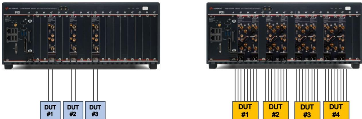
Examples of multi-site measurement configurations
