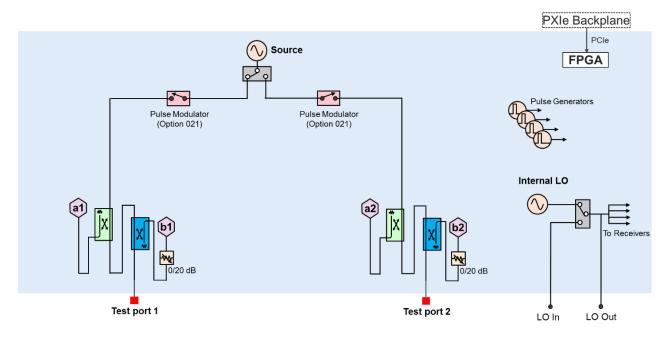
M981xA PXIe Receiver Moule (2-receivers)
