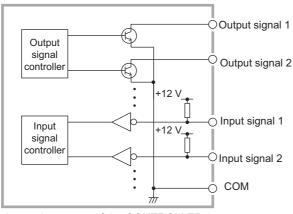
Internal structure of the CONTROLLER
