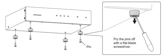
Pry off the pins holding the legs (four locations) with a flat-blade screwdriver.
