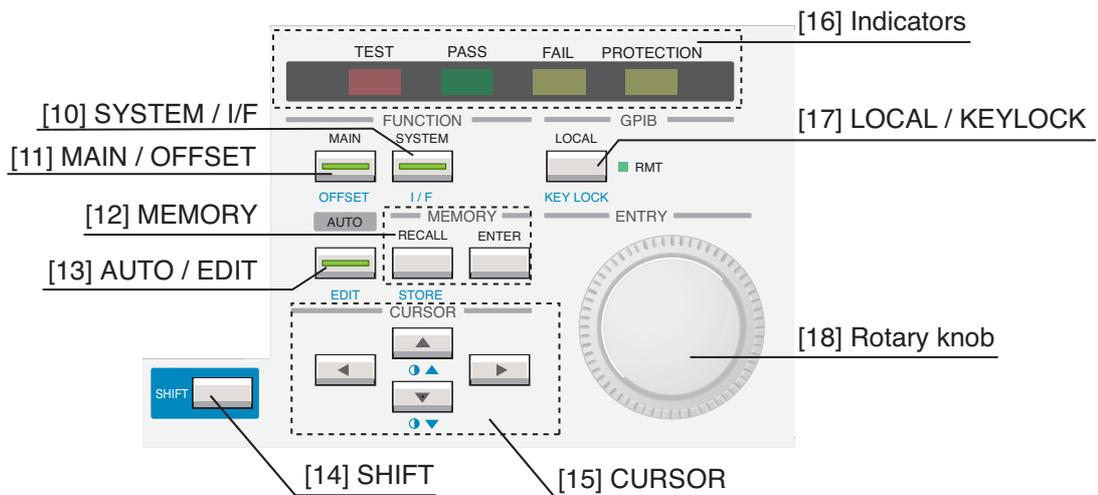
Fig. 3-2 Setup keys (example of TOS6210)
