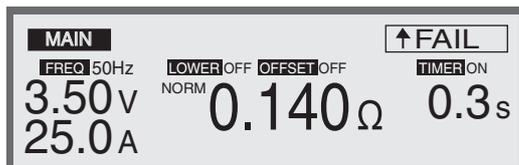
The "↓ FAIL" appears in the upper right part of the LCD when the measured value is below the lower reference value, and the "↑ FAIL" appears in the same part of the LCD when the measured value is above the upper reference value. The FAIL LED indicator also lights, and the buzzer sounds.
