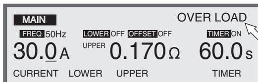
For example, when the test current of TOS6200A is 30 A, if the load resistance (including the resistance of the DUT, the test leads, and any other associated items) from the perspective of the output terminals exceeds  $0.166 \Omega (\cong 150/30^2)$ , the output power exceeds 150 VA, causing an overload. This disables testing.
