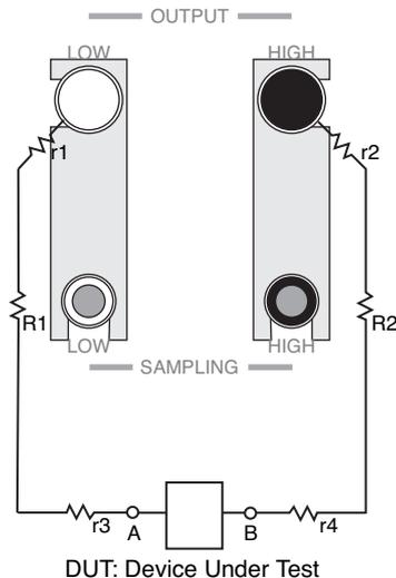
Install the short-circuit bars between the OUTPUT and SAMPLING terminals and connect the leads. The tester measures the total resistance value of contact resistance r1 to r4, resistance components R1 and R2 of the leads, and the resistance between A and B.
