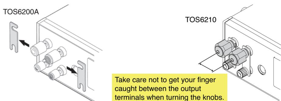
2. Connect the current output line on the crimp terminal side of the test lead (black or white) to the LOW side of the OUTPUT terminals; connect the voltage measurement line on the banana plug side to the LOW side of the SAMPLING terminals. Check that the connections are secure.
