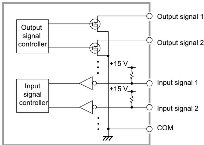
Fig. 5-4 Internal Configuration of the SIGNAL I/O Connector
