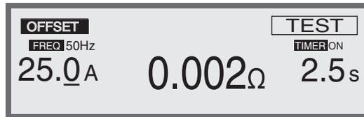
When you press the STOP switch or when the time set in the timer elapses, the tester stores the offset value of that time in memory. When offset measurement ends, the tester reverts to ready status.
