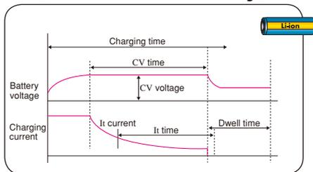
[Termination conditions] Time, CV time, current, and temperature
