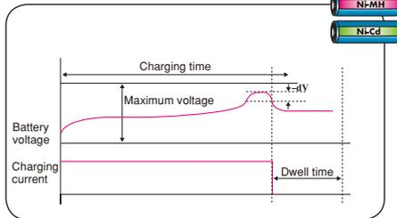
[Termination conditions] Time, voltage,  $-\Delta V$ , temperature, and  $\Delta T/\Delta t$
