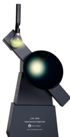
LSG-2000CCD Goniospectroradiometer with Moving Mirror
