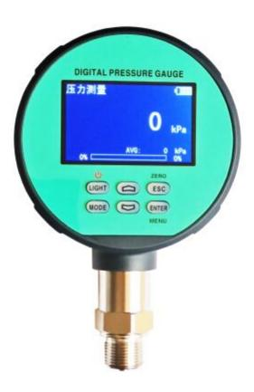
The high-precision digital piezometer has the function of pressure measurement and high accuracy. It can verify pressure transmitter, pressure switch and pressure gauge. It can communicate with computer through RS232 to realize remote control, data processing and printing verification record.
