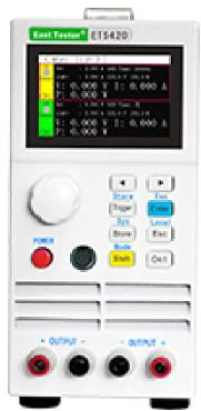
ET54 series single/double channel programmable dc electronic load, USES the high performance chip, high speed, high precision design, provide 1mV, 1mA resolution, superior performance, can be widely applied to the charger, switching power supply, linear power supply, production test of all kinds of batteries and other industries, scientific research institutions such asthe test research and development.
