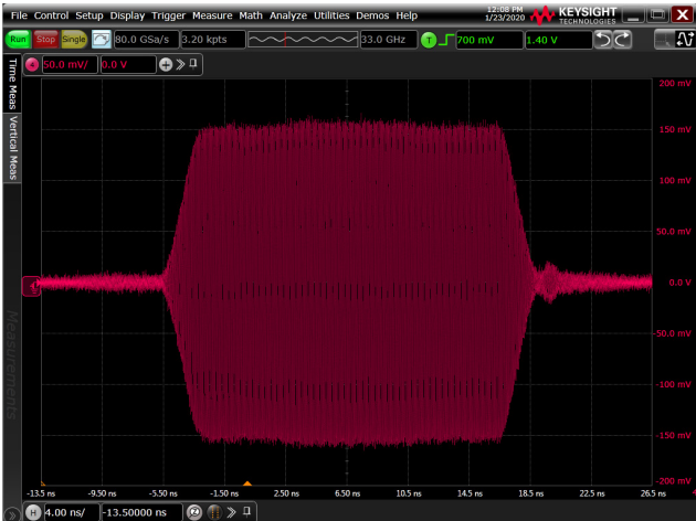
Figure 12. 20 ns pulse with 2 ns rise/fall times.
