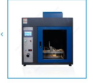
ZRS-3H Glow-wire Test Apparatus
