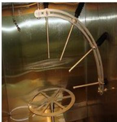
Fig 1: IPX9K nozzle angle diagram
