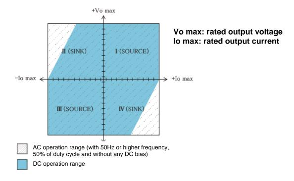
Please avoid continuous use in high frequency. It increases internal loss and leads to being in failure.
