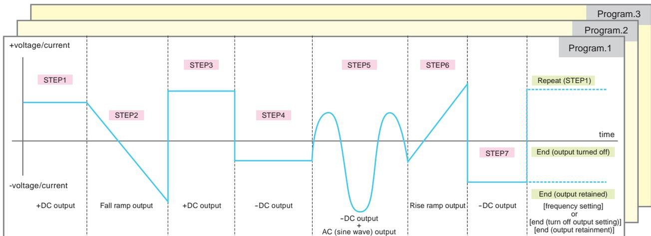
Complicated waveforms such as below can be easily generated just by using the sequence function.
