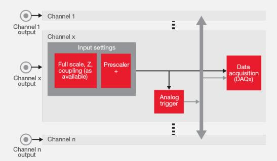
Figure 1. M3102A input functional block diagram, all channels have identical input structure
