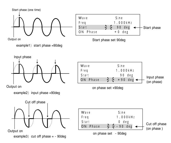
if you set the phase at 180deg, you get negative half wave of sine wave, and also set the phase at -180deg, you get positive half wave.
