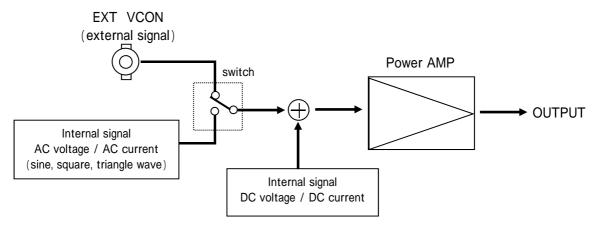
When external signal is active, "EXT VCON" LED(green) is light on, on the contrary, internal signal is active, "EXT VCON" LED(green) is light off.
