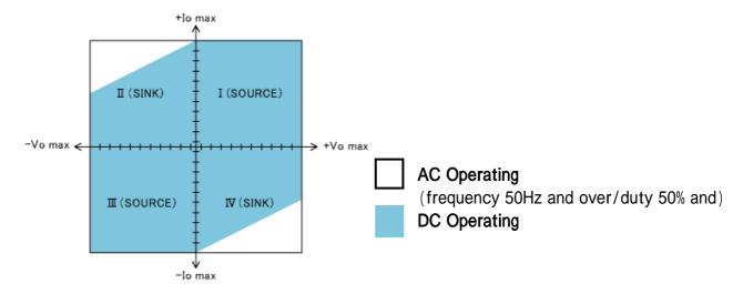
Please avoid continuous use in high frequency. It increases internal loss and leads to being in failure.
