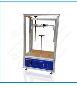
WDT-1 Wire Damaged Tester
