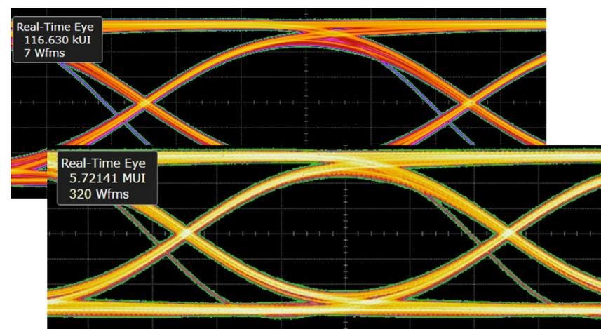
The Infiniium EXR-Series builds eye diagrams 50 times faster than the S-Series. In the same amount of time, the EXR-Series captures 5.7 million UI while the S-Series captures only 0.12 million UI
