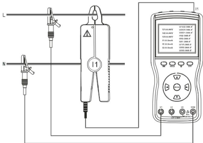
2. Three-phase Four-Wire Voltage, Current, Phase Angle and Sequence, Frequency, Power and Power Factor Measurement:
