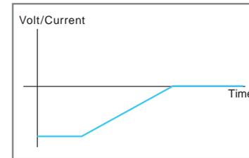
■ Applications: Power activation test, various start-up tests of motor, etc, fluctuation test of wave shape and so on.
