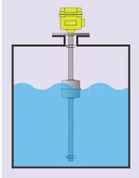
When the liquid level goes Up to reach the START point, the START indicator turns on. At the same time, the START contact signal activates the connected pump.
