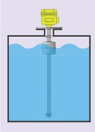
When the liquid level goes Up to reach the HIGH/A point, the HIGH/A indcator turns on. At the same time, the HIGH/A contact signal activates the connected buzzer and purmp.
