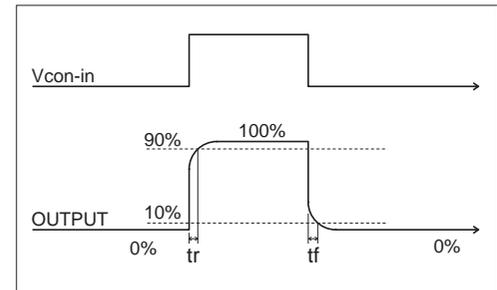
**Response speed:** When accurate output wave is required, please select an amplifier in sufficiently higher frequency band than applied one. Generally, speedy frequency band as 3 to 5 times of applied frequency for sine wave and 10 times for rectangular wave are required. If frequency band is in lacking, as not only output amplitude is reduced but also phase difference between input and output become larger, consideration to utilize it monitoring output wave is required.
