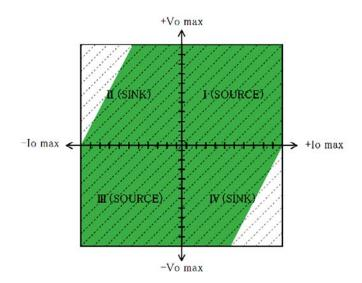
Vo max : Rated output voltage Io max : Rated output current
