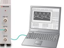
If a different output is used instead of DC, 0 V and 0 A will be displayed since the unit is dedicated to displaying DC output in DJOP series.
