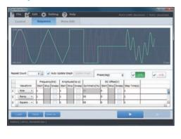
The series features the independent sequence outputs with Ch1 and Ch2. Also, during the sequence operation, you can use the waveform made by a dedicated editor. (As for the waveform of your choice, select one waveform that is commonly used in Ch1 and Ch2.)
