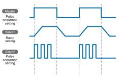
Note The operation accuracy of the timer when sequensing is 0.5%. Be careful when you use it by the long-term running operation.
