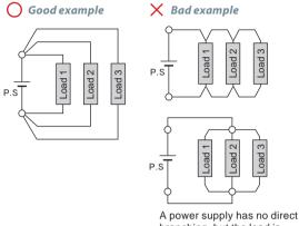
branching, but the load is branched using cables.
