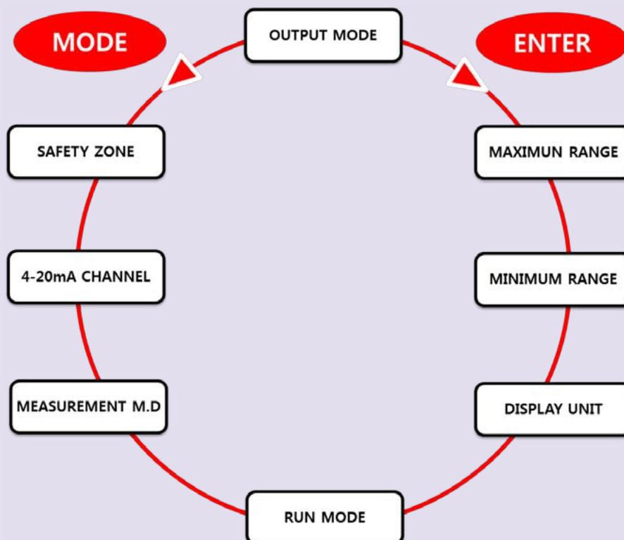
In the menu setting, if press [MODE], it turns counter-clockwise, if press [ENTER], it turns clockwise. With [UP]/[DOWN] key, you can change the value.
