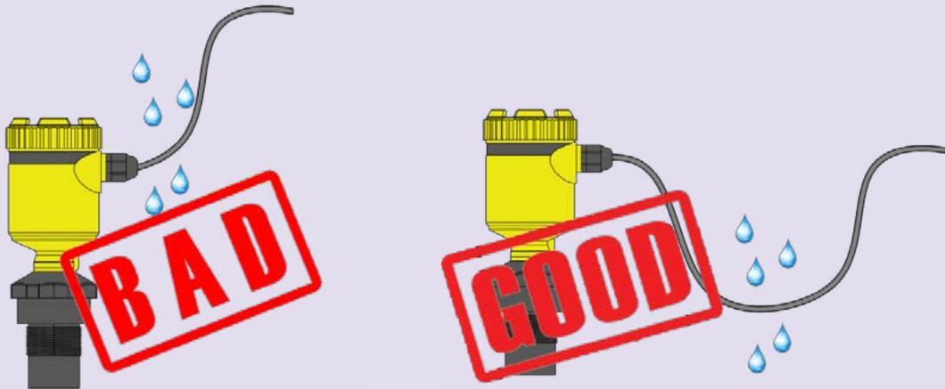
As shown in the above pictures, slacken the cable to the bottom in order to prevent water (rain, any liquid) coming in through the cable gland.
