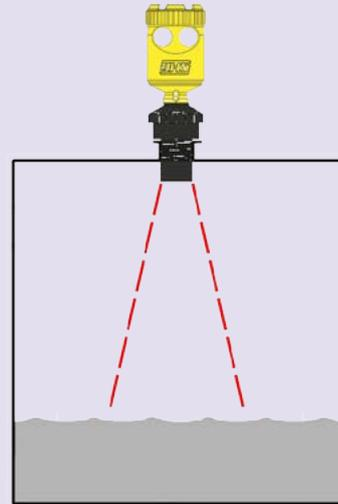
**\* Water drops on the top of the tank can cause sensor malfunction.**
