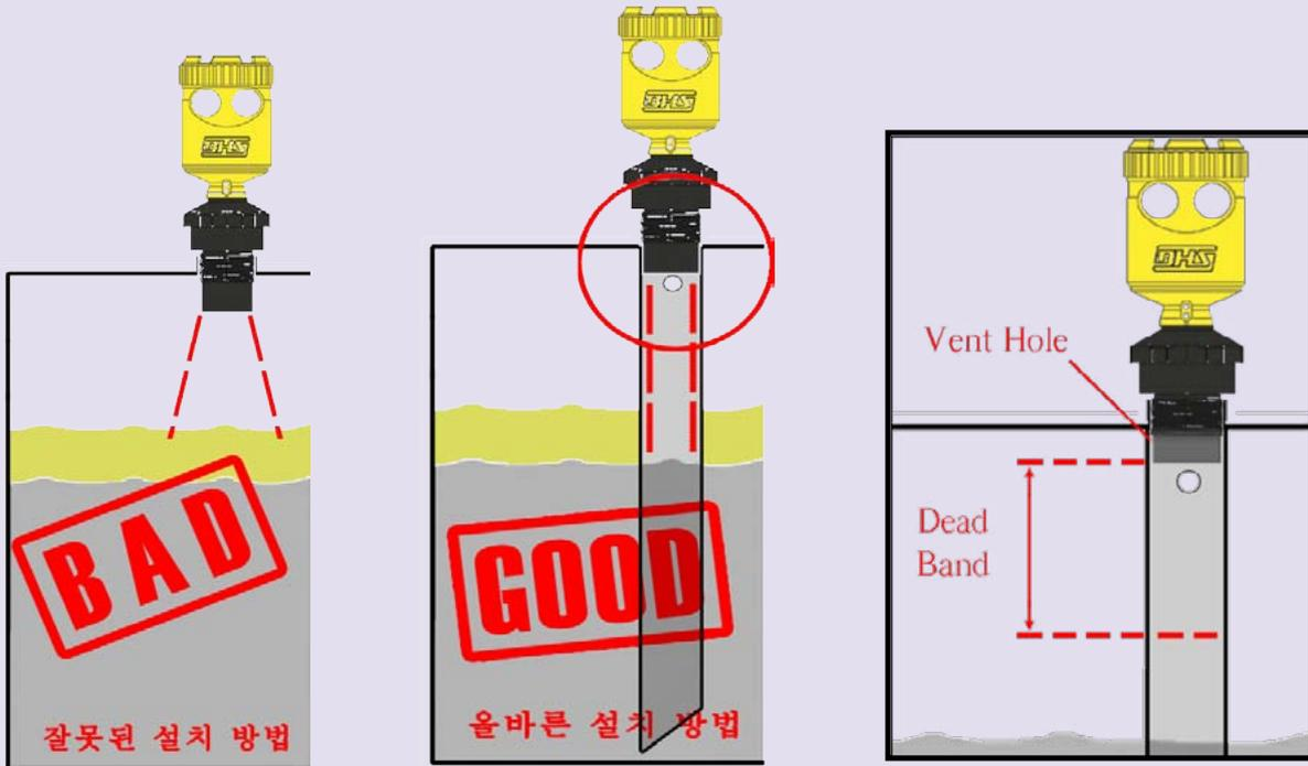
You can prevent malfunction with protection pipe when suspended solid exist in the tank as shown in the above pictures.
