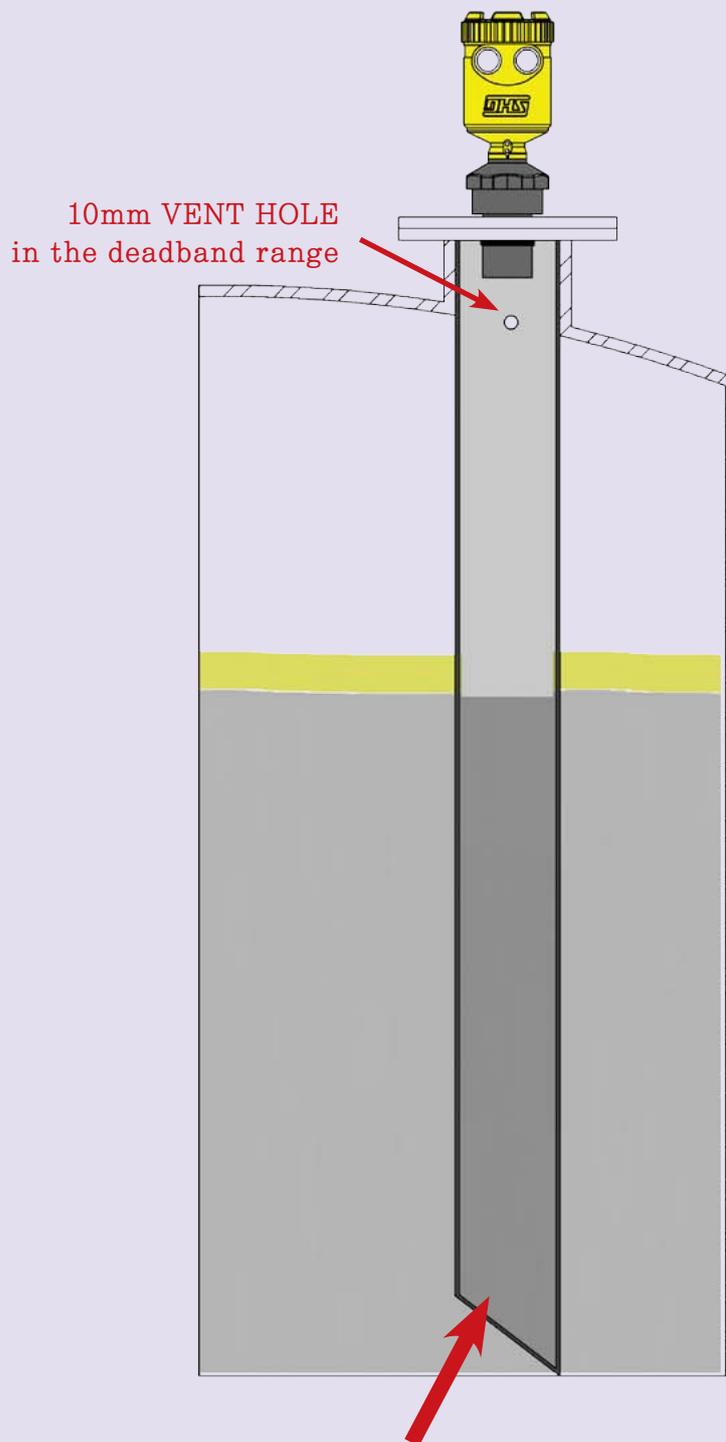
So as to cut into the bottom 15 ~ 45° float in the pipe it is not flowing net installed,
