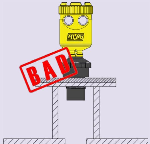
If there is a burr or a welding seam in the inner wall surface of the nozzle it can be recognized in detection target. After installation, you must remove.
