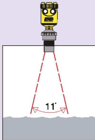
Beamwidth is about 11°. Considering this beamwidth, install the sensor securing enough distance from the wall.
