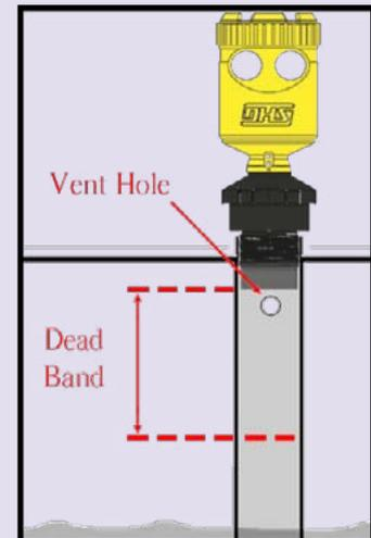
If there are water drops on the top of the tank, be cautious not to affect the sensor beaming. Swell due to water drops can occur sensor malfunction.
