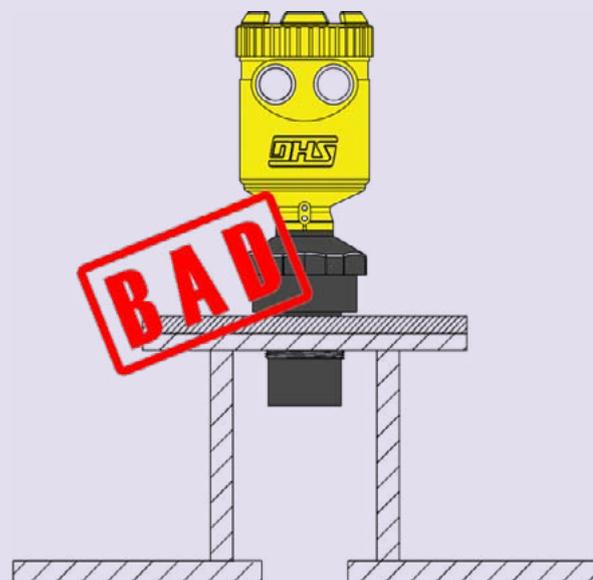
If there is a burr or a welding seam in the inner wall surface of the nozzle it can be recognized in detection target. After installation, you must remove.
