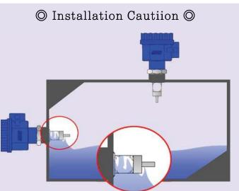
You should pay attention to the phenomenon when using for adhesive liquid, as shown in the picture. A malfunction is caused by the liquid attached to the sensing part.
