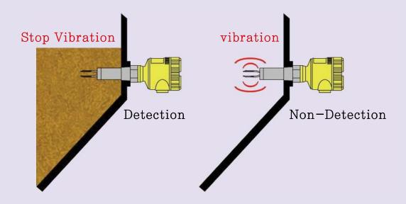
Using in the strong adhesive liquid will cause a malfunction of the sensor. If if impacts on the detecting part, it will cause a malfunction of the sensor.
