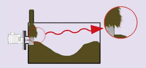
When it prevents the smooth rotation of the pedals, sensors can be mistaken for a malfunction as detecting a large amount of powder.
