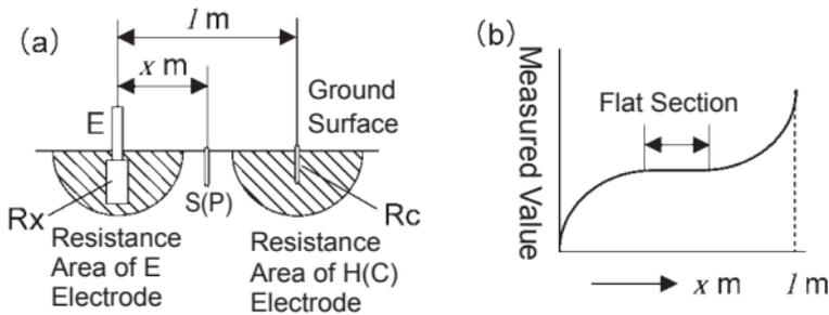
The distance between E-H(C) of the instrument can be up to 50 m by using the optional L9843-51 and L9843-52. In principle, it is possible to carry out measurement even if the distance is more than 50 m. However, the measurement result cannot be guaranteed.
