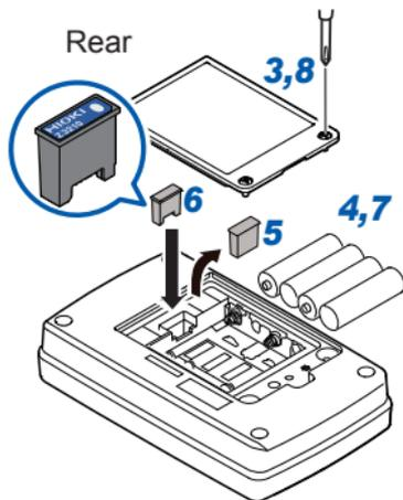
Use a flat-head screwdriver or other suitable tool to remove the Z3210.
