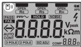
To toggle the wireless communications function on and off, press and hold the **Fn** button and the **COMP** button for at least 1 s.
