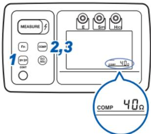
**1** Press the **3P/2P** button to set to **3 POLE** (3-pole method), or **2 POLE** (2-pole method).
