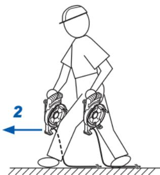
**1** Use the measurement cable (black) to connect between earthing electrode and E terminal.
